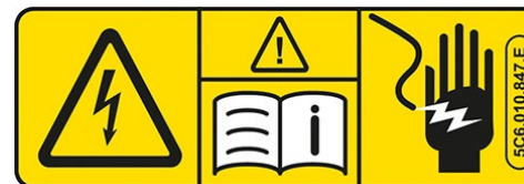
Examples of warning stickers in high-voltage vehicles:
